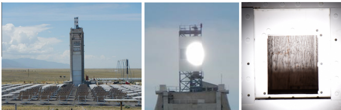
Fig. 3. On-sun testing of a falling particle receiver at the National Solar Thermal Test Facility at Sandia National Laboratories, Albuquerque, NM.
