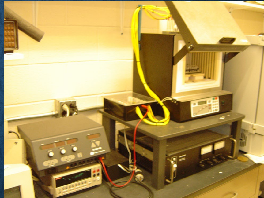
HALT system designed and built at Penn State University
