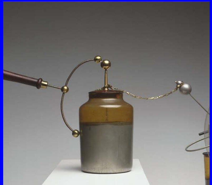
The Leyden Jar: The first Capacitor!
