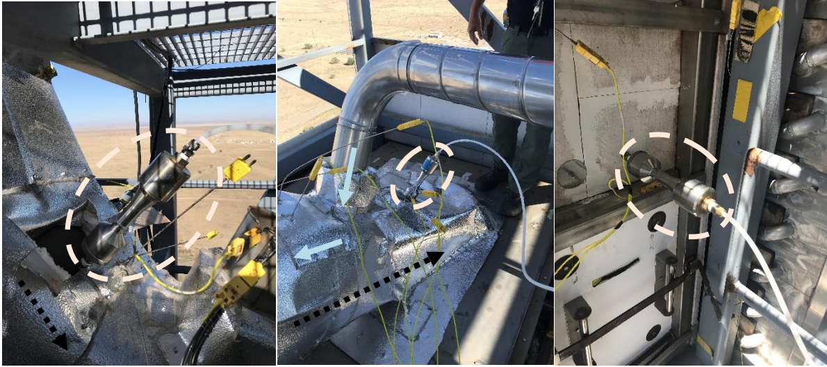
FIGURE 3. Anderson impactors at various locations during the first dust removal study: Top of chute/before dust removal loop (Left), bottom of chute/after dust removal loop (Middle), receiver (Right) with the particle flow direction shown by the black dotted lines and the air flow direction shown by the solid blue lines.
