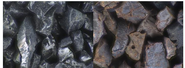
FIGURE 5: WANLI DIAMOND BLACK PARTICLES AS-RECEIVED (LEFT) AND AFTER 10,000 CYCLE WITH A PEAK CYCLE TEMPERATURE OF 975 °C (RIGHT)
