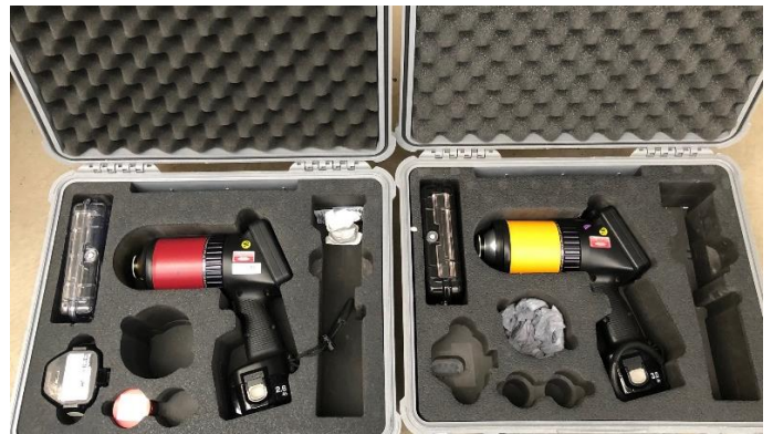
FIGURE 3: SOLAR 410 REFLECTOMETER AND ET 100 EMISSOMETER
