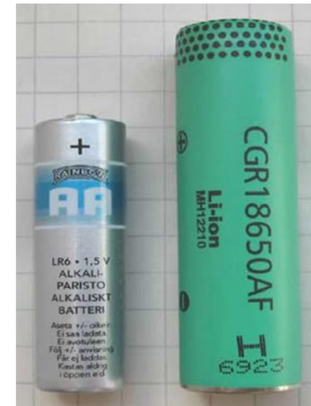
18650 cell format used in 85 kWh Tesla battery
