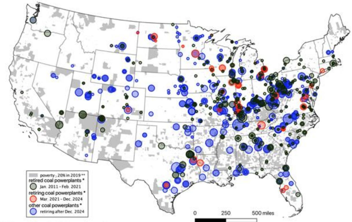
\* circles are scaled based on the EIA's nameplate capacity
