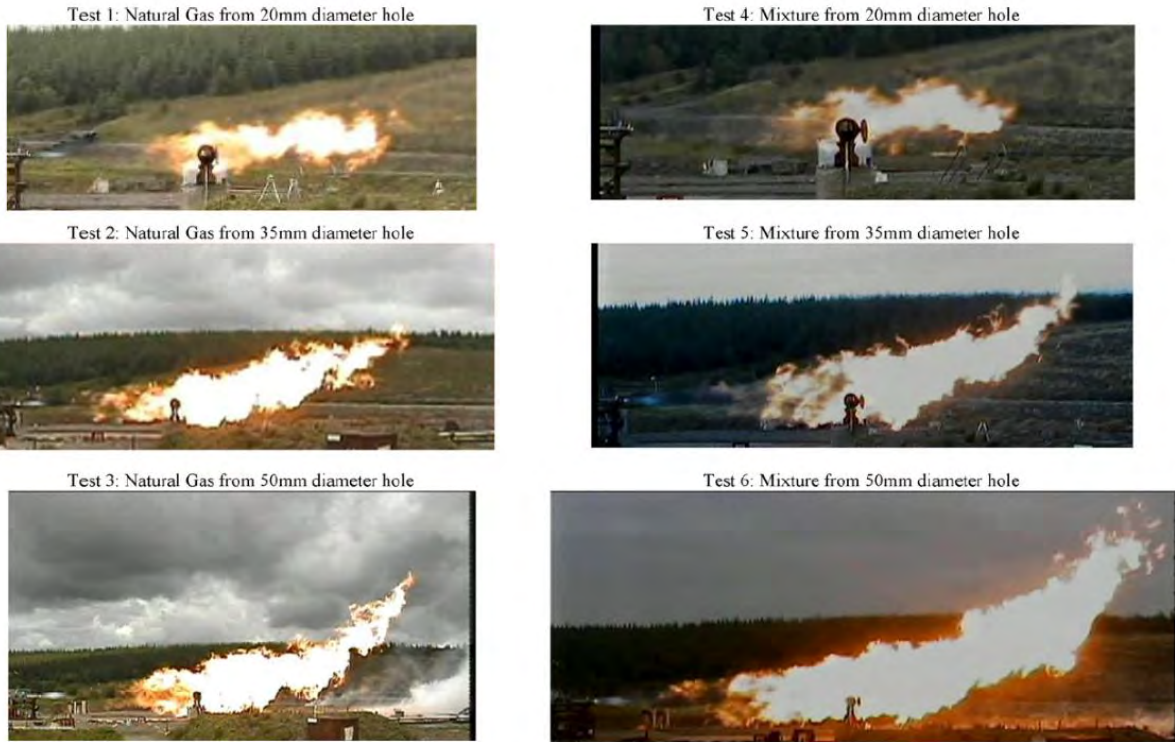
Figure 2-16. Jet Flame in Test Images (not all the same scale) (from [18])
