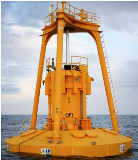
FIGURE 1. OCEAN POWER TECHNOLOGIES' POWER BUOY OPERATING OFF THE COAST OF SCOTLAND. THE WETTED SURFACE AREA AND ORIENTATION OF THE DEVICE REMAIN APPROXIMATELY CONSTANT AS THE BUOY REACTS TO ONCOMING WAVES, ALLOWING THE POWER BUOY TO BE EFFECTIVELY MODELED USING LINEAR HYDRODYNAMICS METHODS. PHOTO FROM OCEAN POWER TECHNOLOGIES, NREL 22857
