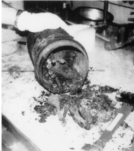
Figure 3: Excessive corrosion after 30 day test at 725°C with Ar-10% O 2 as the ullage gas [16].
