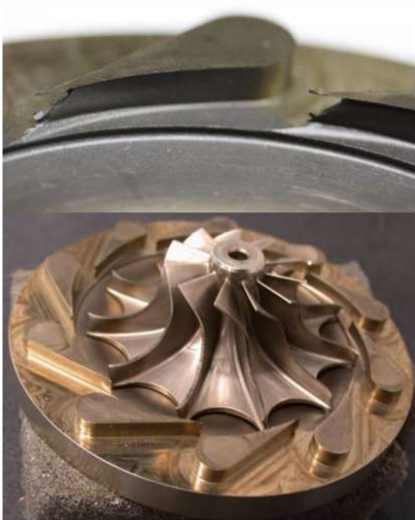
Figure 3-1: Turbine nozzle with substantial amount of erosion, and turbine wheel with placement inside turbine nozzle.
