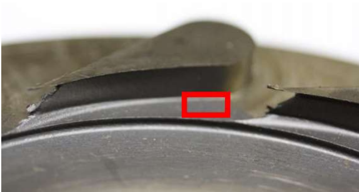
Figure 4-1: Turbine Nozzle with undercut and the EDS sample location represented by red square
