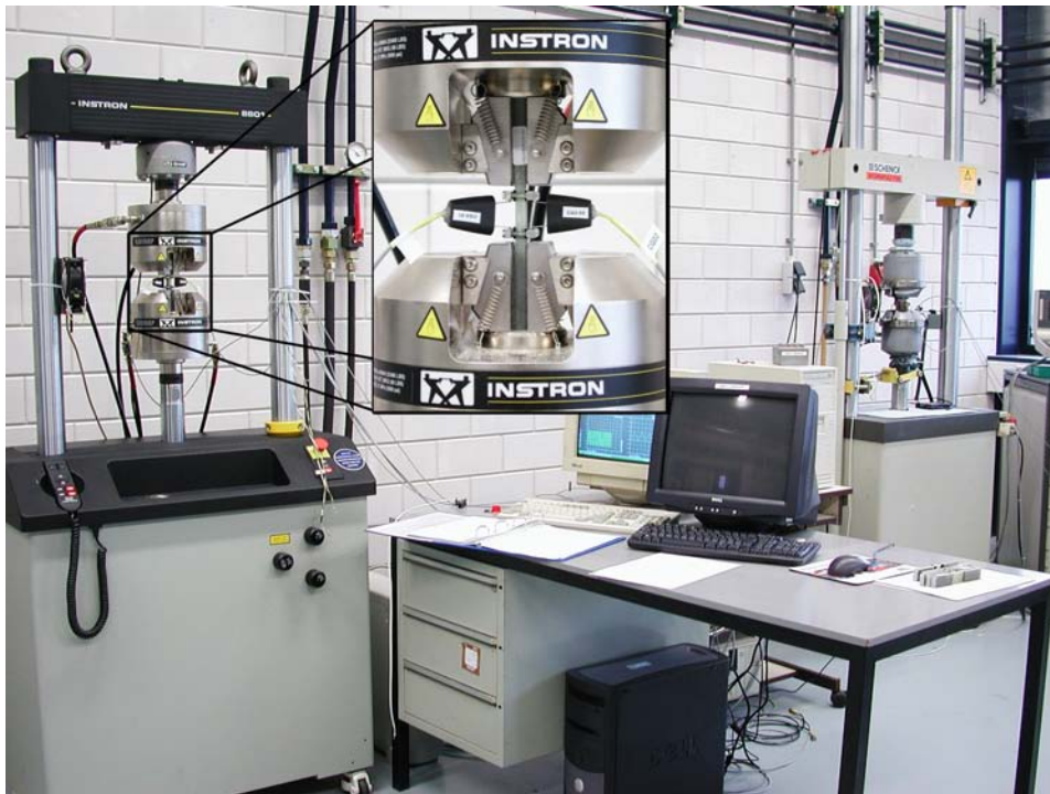
Figure 57: Representative OPTIMAT test-set up at WMC
