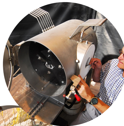
The CR5 device (left) contains the counter-rotating ceramic rings. The solar energy from the concentrator passes through the aperture (hole in the white disk in front of Rich Diver) and onto the reactive rings. Above, the CR5 device is in place at the solar furnace. The parabolic reflector of segmented mirrors can concentrate the sun's energy up to 6750 times ambient solar radiation—the CR5 easily achieves ~1500 °C on the reactive rings.
