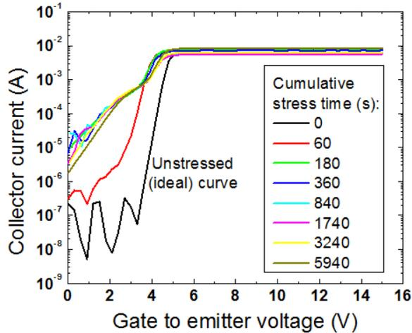
**Figure 3.**  $I_C$ - $V_{CE}$  curves resulting from stressing an IGBT at  $V_{GE} = 20$  V,  $V_{CE} = 2$  V ( $I_C \approx 38$  A), corresponding to a condition of high electric field in the gate oxide and moderate thermal stress.
