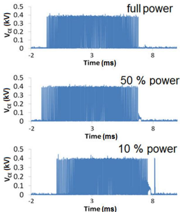
**Figure 8. Collector-emitter waveforms for an IGBT monitored *in situ* for an inverter operating at (1) 100% of rated power, (2) 50% of rated power, and (3) 10% of rated power.**
