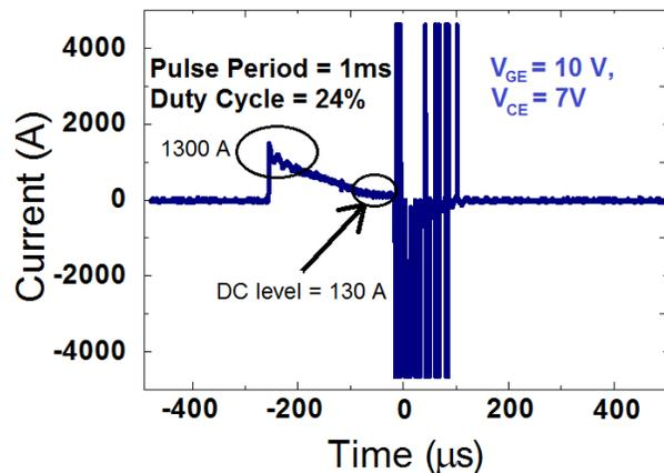
**Figure 5.** IGBT collector current resulting from pulsed gate input. Measurement is made at room temperature.
