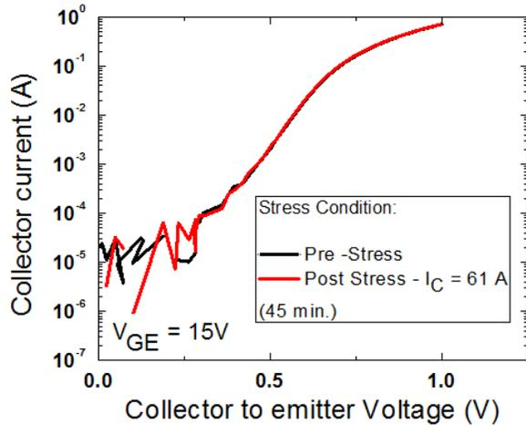
**Figure 1. Pre and post-stress  $I_C$ - $V_{CE}$  curves for typical IGBTs, after 45 min stress at  $I_C \approx 61$  A.**
