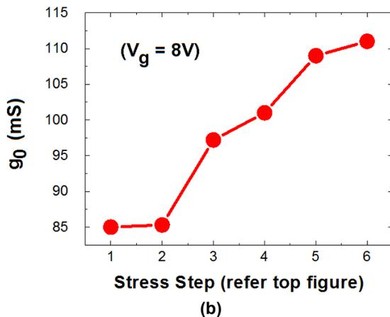
**Figure 6. (a) DC  $I_C$ - $V_{CE}$  curves for an IGBT subjected to increasing increments of AC stress. (b) The output conductance ( $g_0$ ) measured at the end-point of each of the curves in the top portion of the figure ( $V_{GE} = 8$  V,  $V_{CE} = 15$  V) for each of the steps in the sequence.**
