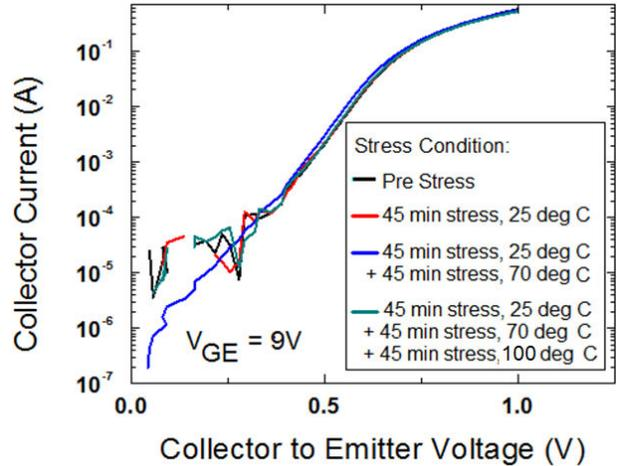
**Figure 2. Pre- and post-stress  $I_C$ - $V_{CE}$  curves for a typical IGBT with stress temperatures of 25, 70 and 100°C for 45 min. each.**
