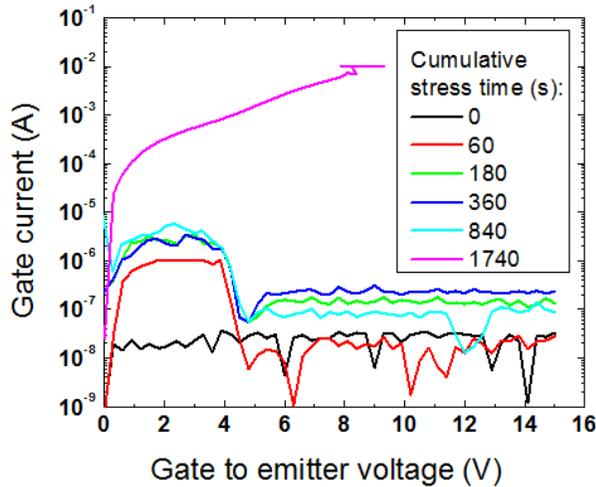
**Figure 4.**  $I_G$ - $V_{CE}$  curves resulting from stressing an IGBT at  $V_{GE} = 20$  V,  $V_{CE} = 2$  V ( $I_C \approx 38$  A), corresponding to a condition of high electric field in the gate oxide and moderate thermal stress.
