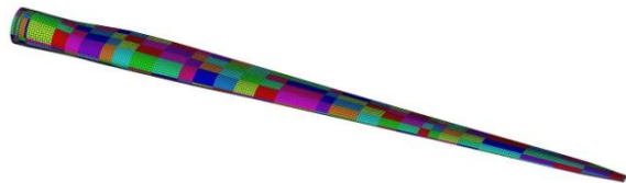
Figure 3. ANSYS finite element mesh for SNL 5-MW blade model
