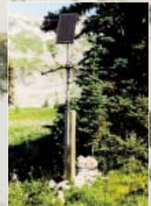
▽ The Pacific Northwest Seismograph Network maintains many photovoltaic-powered monitoring stations like the one shown here on Mt. Rainier, Washington, where seismic data are collected and transmitted to assist in forewarning about earthquakes and volcanoes. [Photo courtesy Pacific Northwest Seismograph Network]
