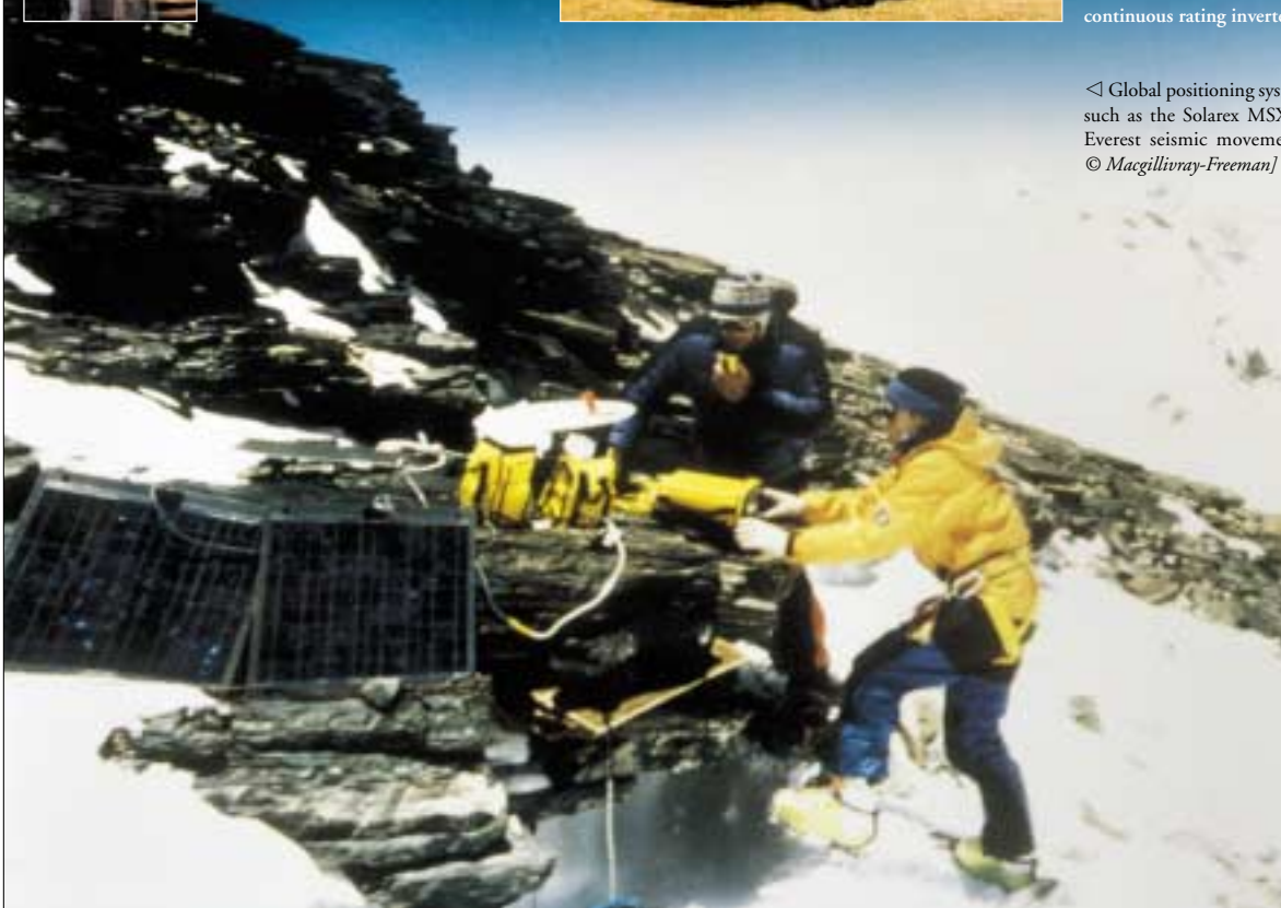
▽ The Pacific Northwest Seismograph Network maintains many photovoltaic-powered monitoring stations like the one shown here on Mt. Rainier, Washington, where seismic data are collected and transmitted to assist in forewarning about earthquakes and volcanoes. [Photo courtesy Pacific Northwest Seismograph Network]
