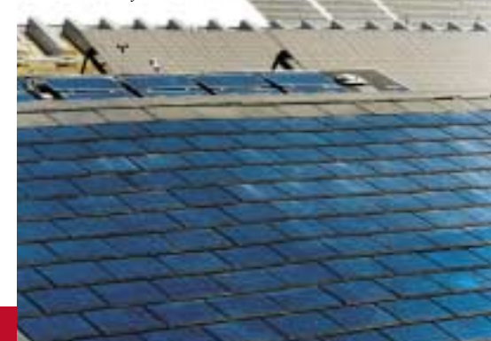
▽ At a California PVUSA site, this roofing shingle test bed allows more successful residential grid-tied installations throughout the U.S. [Photo courtesy PVUSA]
