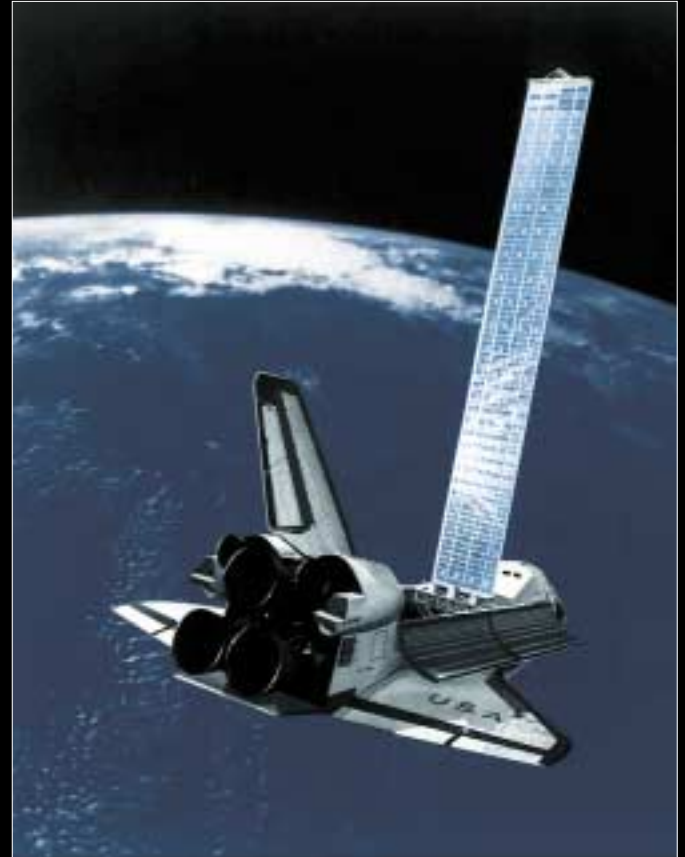
△ Photovoltaic cells were first used in space to power a 5mW backup transmitter on the Vanguard 1 in 1958. Sputnik used PV. Indeed, solar cells power most satellites in space today, and the U.S. shuttle fleet uses PV to generate much of its electrical power [Photo courtesy National Renewable Energy Laboratory from a Lockheed rendition]
