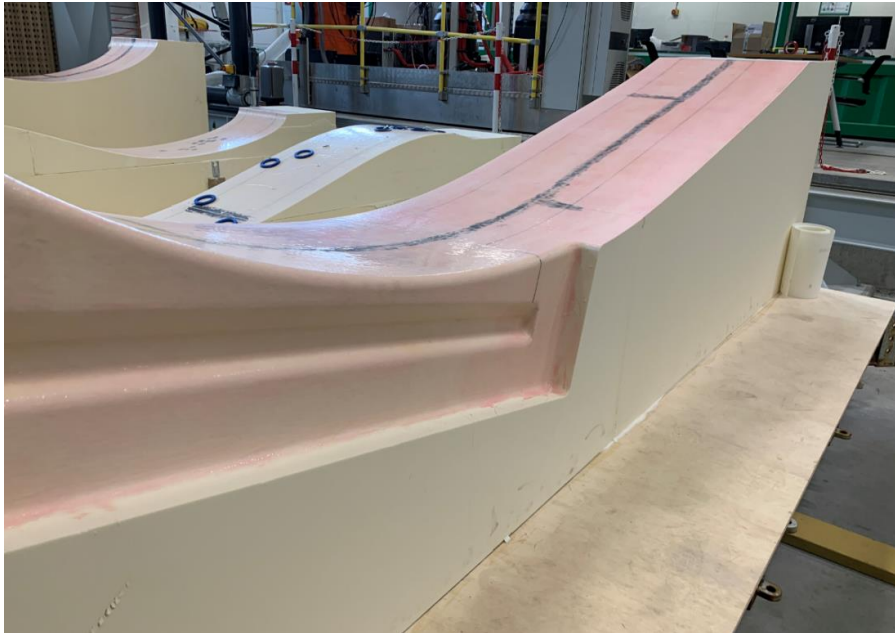
Molds for pressure shells in the Fraunhofer IWES demo center, milled from foam blocks with epoxy coating.
