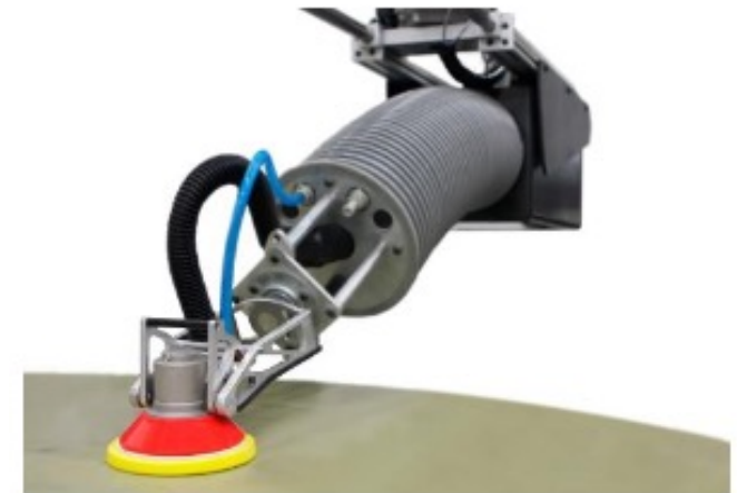
Temple Allen EMMA® robotic sand, grind, polish robot.
