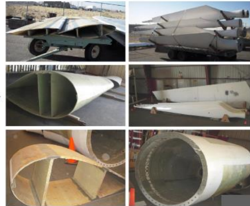
Figure 3-7: Wind Turbine Blade Test Specimen Library – Actual Airfoil and Blade Root Sections Representing Multiple Blade Sizes, Manufacturers and Construction Types
