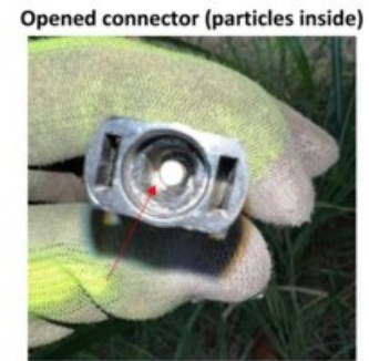
Visible debris or foreign particle inside connector body
