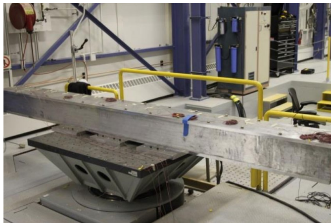
Figure 1. Surrogate assembly in the 1 DOF shake table test
