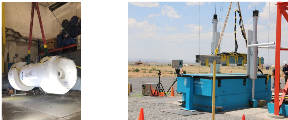
Figure 13. 30 cm drop test with 1/3 scale cask (left) and surrogate fuel assembly (right).
