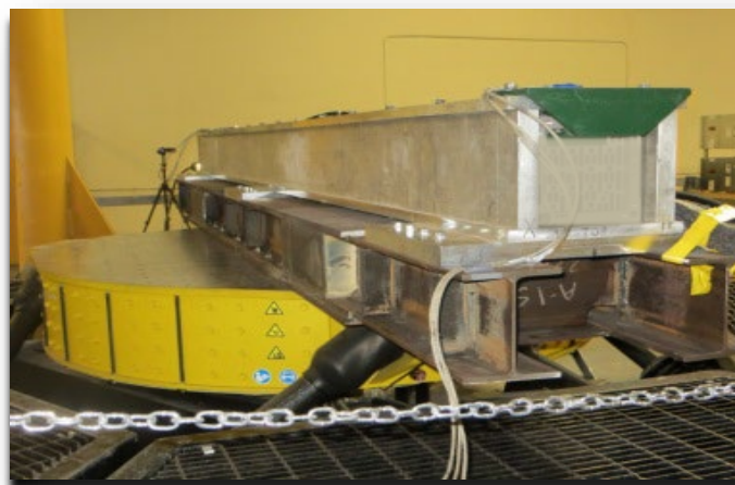
Figure 3. Surrogate Assembly in the 6 DOF shake table test
