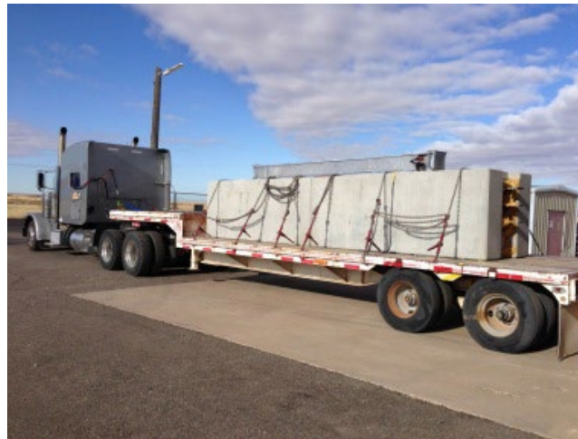
Figure 2. Surrogate Assembly in the over-the-road truck transport test
