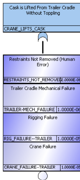
Figure 10-4. Fault tree 3.1, cask is lifted from trailer cradle without toppling.
