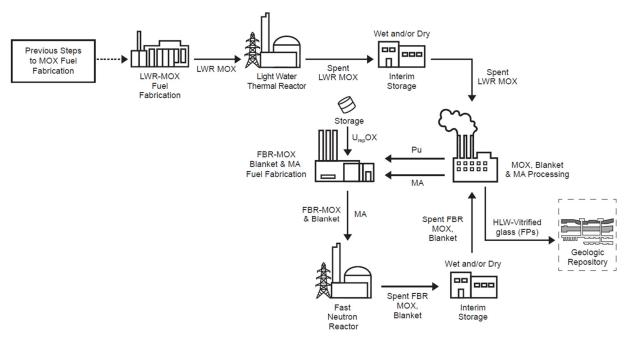
**FIGURE 4.9** Schematic diagram of the fuel cycle that combines LWRs and fast reactors for multirecycling Pu and partitioning and transmuting minor actinides. If the fast reactor in the diagram is operating as a burner (CR <1), there would be no need for blanket fuel. Blanket fuel is required for breeding (where more fissile material is produced than consumed).
