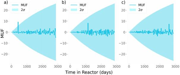
**FIGURE 6.1** The average measurements of material unaccounted for (MUF) as a function of the time fuel spends in the reactor for the three loss scenarios: (a) early lifetime loss, (b) midlifetime loss, and (c) end of lifetime loss. SOURCE: Higgins et al. (2021). Courtesy of Sandia National Laboratories.
