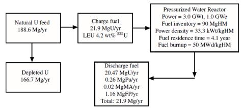
**FIGURE E.2** Material flow for a pressurized water reactor design with once-through low-enrichment uranium (LEU) fuel.
