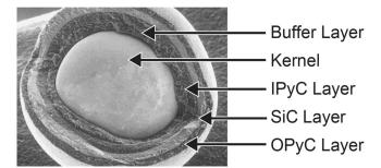
**FIGURE G.2** Cross section of TRIstructural ISOtropic (TRISO) fuel particle, showing fuel kernel encased in buffer, pyrolytic carbon (IPyC and OPyC), and silicon carbide (SiC) layers. SOURCE: Idaho National Laboratory.
