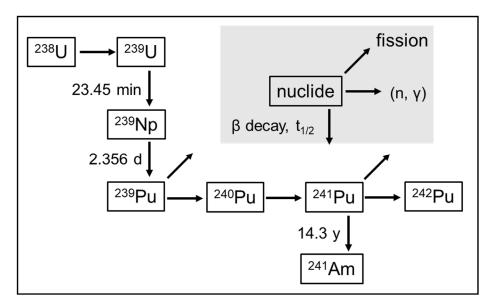
**FIGURE 3.3** Successive capture  $(n,\gamma)$ /fission/beta decay reactions originating from a single radionuclide, illustrating generation pathways for the production and destruction of Pu isotopes from the reaction of  $^{238}$ U with neutrons.
