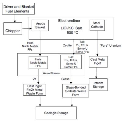
**FIGURE 4.11** Schematic of pyroelectrometallurgical treatment used for metallic fuel for the Experimental Breeder Reactor II. Block diagram with (left) and without (right) the cadmium electrode. "Pure" uranium in the diagram denotes uranium that is relatively pure but requires additional purification steps to reach the desired purity. NOTE: FP = fission product; TRU = transacratic element.
