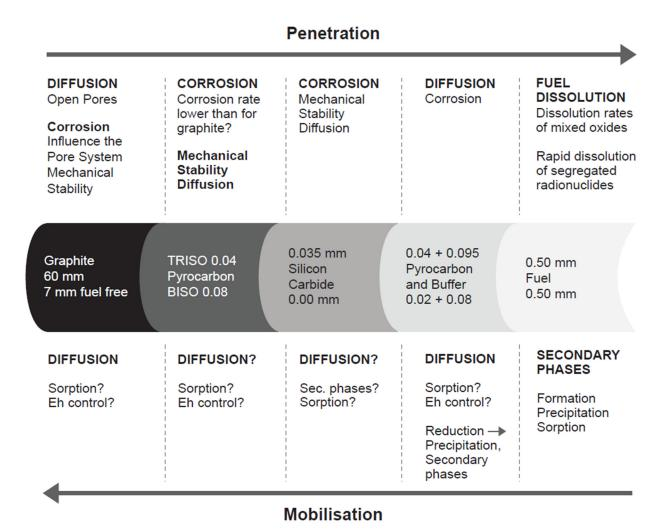
**FIGURE G.1** Penetration of leachants and release of radionuclides for a spent high-temperature reactor TRistructural ISOtropic (TRISO) fuel pebble. The question marks signify issues for which additional research and development is required.
