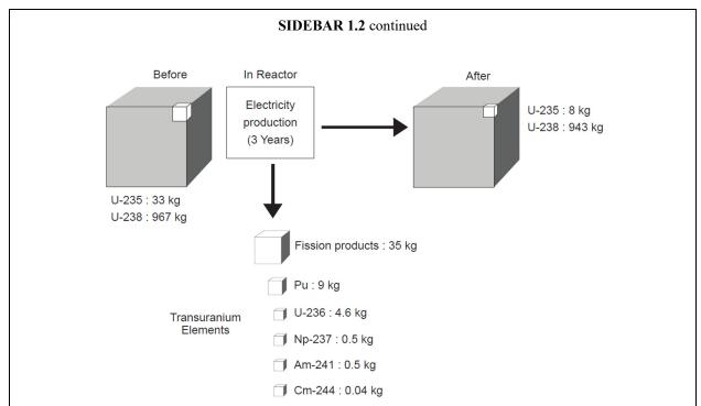
**FIGURE** Typical composition of spent nuclear uranium oxide fuel from a 1000 MWe pressurized water reactor with an initial charge of 1000 kg of U with <sup>235</sup>U enriched to 3.3 percent after roughly 3 years of operation (burnup 33 GWd/MT).
