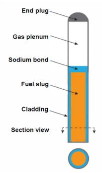
**FIGURE 4.2** Schematic of a typical metallic fuel element sodium bonded to the cladding for improved heat conduction.
