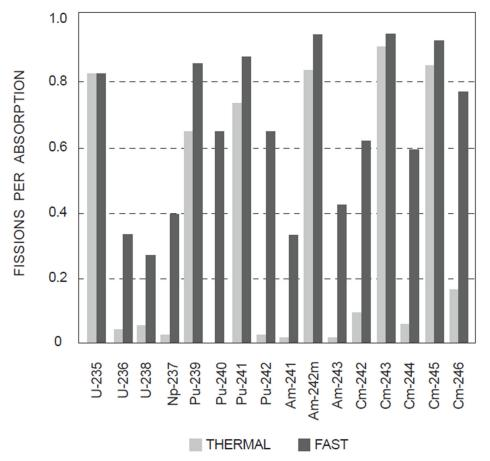
**FIGURE 4.8** Probability of fission per neutron absorbed in actinide isotopes for thermal and fast spectra (e.g., for <sup>239</sup>Pu, probability 0.65 in a thermal spectrum and 0.87 in a fast spectrum). SOURCE: Adapted from Wade and Hill (1997).
