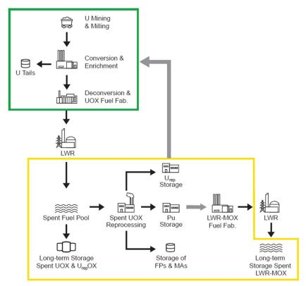
**FIGURE 2.1** Today's LWR fuel cycle components—Established processes and facilities in commercial operation. NOTES: Front- and back-end facilities or operations are highlighted in green and yellow, respectively. FP = fission product; LWR = light water reactor; MA = minor actinides; MOX = mixed oxide; UOX = uranium oxide; Urep = reprocessed uranium.
