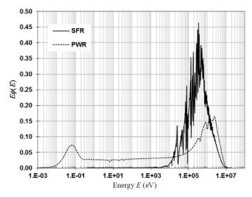
**FIGURE E.1** Comparison of neutron flux spectrum for fast and thermal reactors. NOTE: PWR = pressurized water reactor; SFR = sodium-cooled fast reactor. SOURCE: Lee (2020).
