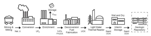
**FIGURE 1.1** Schematic of an open or once-through fuel cycle for a light water reactor (LWR). NOTE: Nat. U = natural uranium;  $U_{dep} = \text{depleted uranium}$ ;  $UF_6 = \text{uranium hexafluoride}$ ; UOX = uranium oxide. SOURCE: Adapted from MIT (2011).
