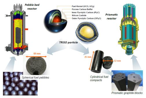
**FIGURE 4.1** Reactor configuration using TRISO fuel particles as pebbles in a pebble-bed reactor or a cylindrical fuel compact embedded in graphite blocks in a prismatic reactor. SOURCE: Adapted from Demkowicz (2019), slide 10.
