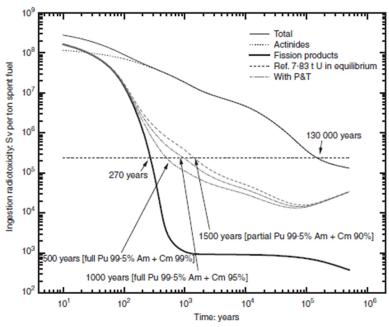
**FIGURE 4.12** Evolution of ingestion radiotoxicity as a function of time for an initial inventory of actinides for fuel with 4.2 percent enrichment, 50GWd/t burnup, and 6 years cooling time. The radiotoxicity reference level (horizontal dashed line) is set at 7.83 MT of natural U, or the amount of natural U required to produce 1 MT of fresh fuel enriched to 4.2% <sup>235</sup>U.
