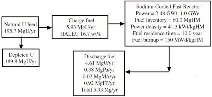
FIGURE E.3 Material flow for a sodium-cooled fast reactor design with once-through high-assay low-enriched uranium fuel (HALEU).
