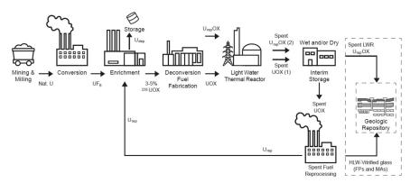
**FIGURE 4.5** Steps in monorecycling uranium (U) in light water reactors (LWRs). Spent UOX (1) refers to the spent fuel resulting from the initial load of UOX fuel. Spent  $U_{rep}OX$  (2) refers to the spent fuel resulting from the initial load of  $U_{rep}OX$  fuel.
