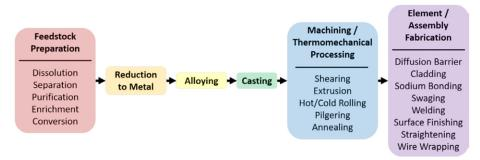
FIGURE 4.3 Process flow for fabrication of metallic fuel.
