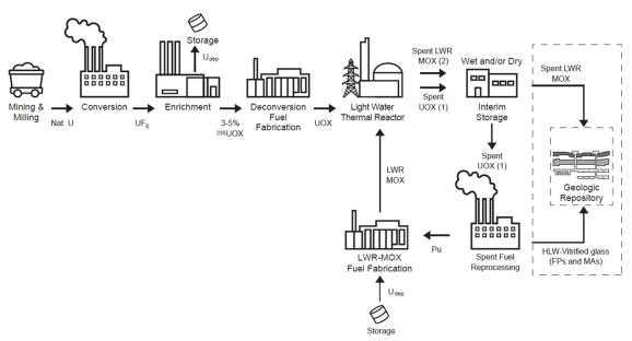
**FIGURE 4.6** Steps for monorecycling Pu fuel in LWRs. Spent UOX (1) refers to the spent fuel resulting for the initial load of UOX fuel. Spent LWR MOX (2) refers to the spent fuel resulting from the initial load of LWR-MOX fuel.
