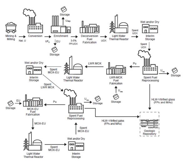
**FIGURE 4.7** Multirecycling of Pu in light water reactors (LWRs) using mixed oxide fuel plus enriched U (MOX-EU).
