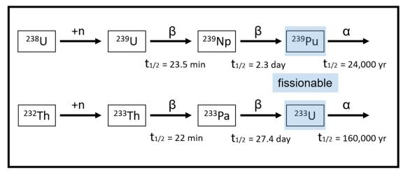
FIGURE 3.2 Pathways for producing <sup>239</sup>Pu from <sup>238</sup>U (top) and <sup>233</sup>U from <sup>232</sup>Th (bottom) by the capture of neutrons.
