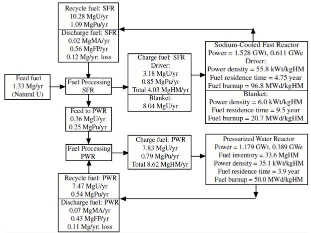
**FIGURE E.6** Material flow for a coupled SFR-PWR system, utilizing Pu-U-Zr fuel for the SFR and U-Pu mixed oxide fuel for the PWR.
