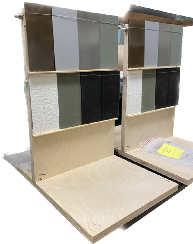
Figure 27. Wooden fixtures used to hold coating specimens in front of the linear ^{60}\text{Co} array at Sandia's Gamma Irradiation Facility. Thin gauge 304 stainless steel wire was used to prevent the specimens from falling into the containment pool and to hold the specimens flat against the fixture during exposure. Samples were wrapped in foil to prevent abrasion against the wire (not shown).
