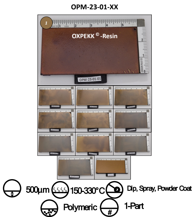
Figure 5. Intake photos of OX-PEKK® coating samples OPM-23-01-01 provided by OPM. Also shown are basic attributes (approximate thickness, cure temperature, application methods, coating type, and number of components). *Note: OPM-23-01-01 was not used as it appears to have cured at a higher temperature, therefore OPM sent OPM-23-01-11. Because there was delay in the receipt of the coatings, OPM-21-01-15 was used in the radiation studies.
