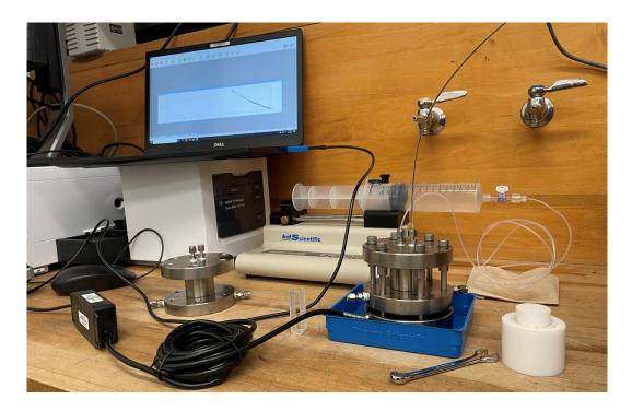
**Figure 7-4.** Bentonite erosion experiment. A 5 mL·hr<sup>-1</sup> flow of deionized water was provided by the syringe pump to the bentonite erosion cell and flowed to a fraction collector located to the right, just out of frame. The load cell measured a swelling pressure logged data to the computer.
