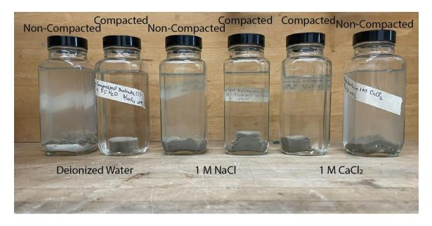
**Figure 7-7.** Bentonite free-swelling experiment after 30 minutes. Compacted and non-compacted forms of bentonite are shown in deionized water, 1 M NaCl, and 1 M CaCl<sub>2</sub>. All bottles contain 10 g of bentonite.
