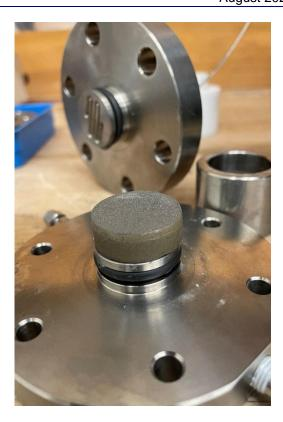
**Figure 7-1.** The bentonite erosion cell. A plug of bentonite is emplaced in the titanium cell and separated from the flow field by a titanium frit. The frit allows bentonite colloids to pass through while the bulk bentonite is retained.
