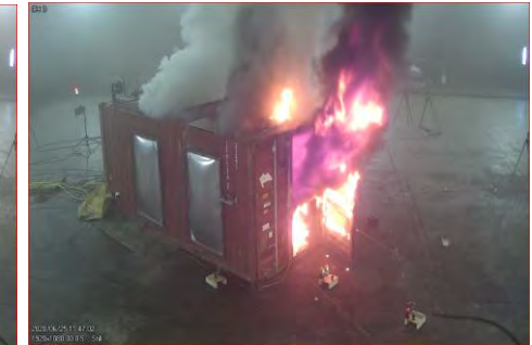
Flashover and flaming from open door [TR + 02:09:48]
