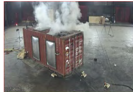
Continued thermal runaway propagation [TR + 00:46:26]
