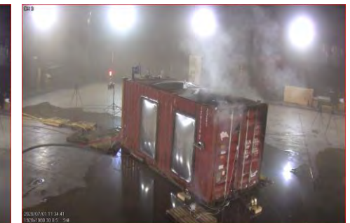
TR propagation continues after water flow restarted [TR + 01:49:54]
