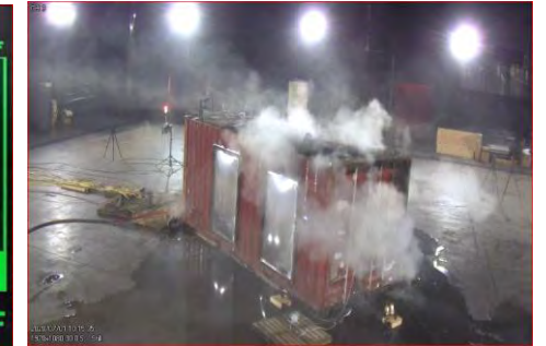
Smoke and gas release from TR propagation [TR + 00:30:49]
