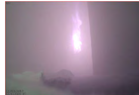
Ignition leading to sustained flaming [TR + 00:08:49]
