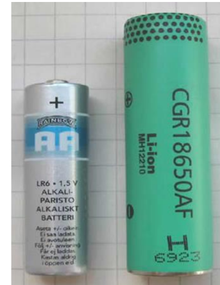
18650 cell format used in 85 kWh Tesla battery
