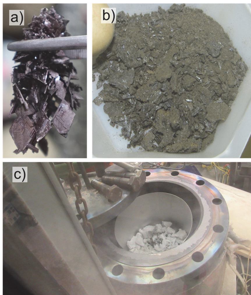
Figure 2. \text{UCl}_3 - \text{NaCl} production. (a) DU dendrites from electrorefining operations, (b) \text{UCl}_3 after distillation and (c) \text{UCl}_3 inside of stainless-steel crucible prior to closing MFIT pressure vessel.
