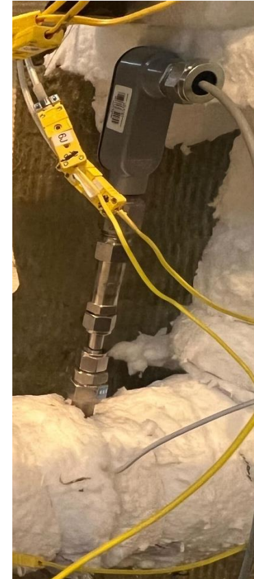
FEES sensors deployed at industrial partner's engineering scale forced convection FLiBe experiment (left). FEES sensor installed in industrial partner's flow loop (right).
