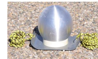
12-inch aluminum sphere (ball drag) simulating a belly crawler
