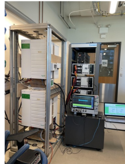
Microgrid PHIL Platform with Hybrid Energy Storages
