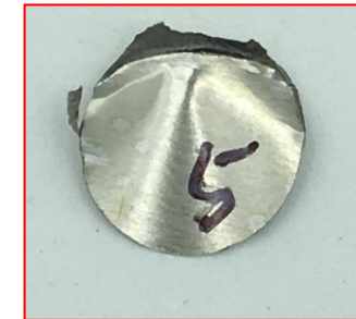
Heavy spur implies the material is too ductile
