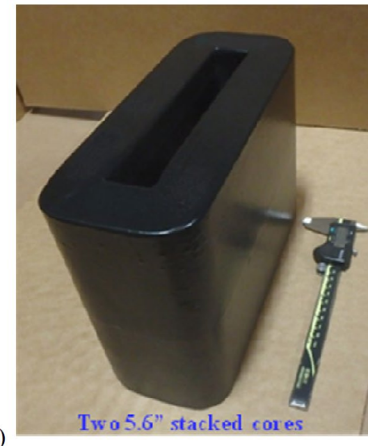
Figure 3: a) Full sized spool of 142mm (5.6") wide FT-3W weighing 500 kgs and b) Inductor core fabricated from the 142mm nanocrystalline FT-3W ribbon.
