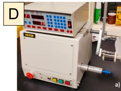
Figure 5. Winding machine to supplement the large-scale fabrication setup.
