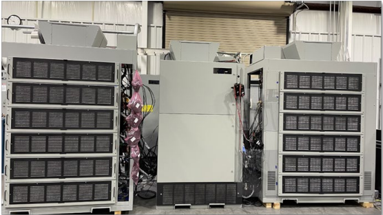
The first SiC based medium voltage Mega-watt industry motor drive product
