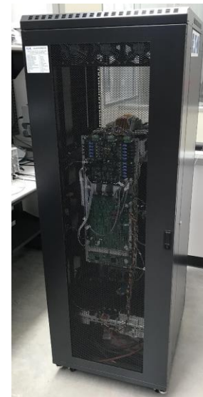
Solid State Transformer (Silicon Carbide Based Power Electronics)
