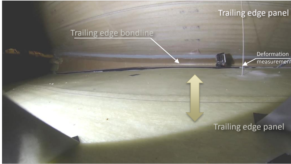
Inside view of the blade towards the trailing edge
