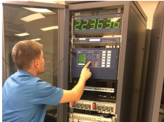
Phasor Measurement Units are used in Sandia's Control & Optimization of Networked Energy Technologies Lab to advance the grid's resiliency and reliability.
