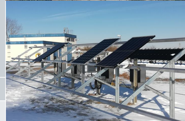
Fig. 2. Solar measurement equipment at two of the test sites: BRA-BTS (top) and GER-BBG (bottom).
