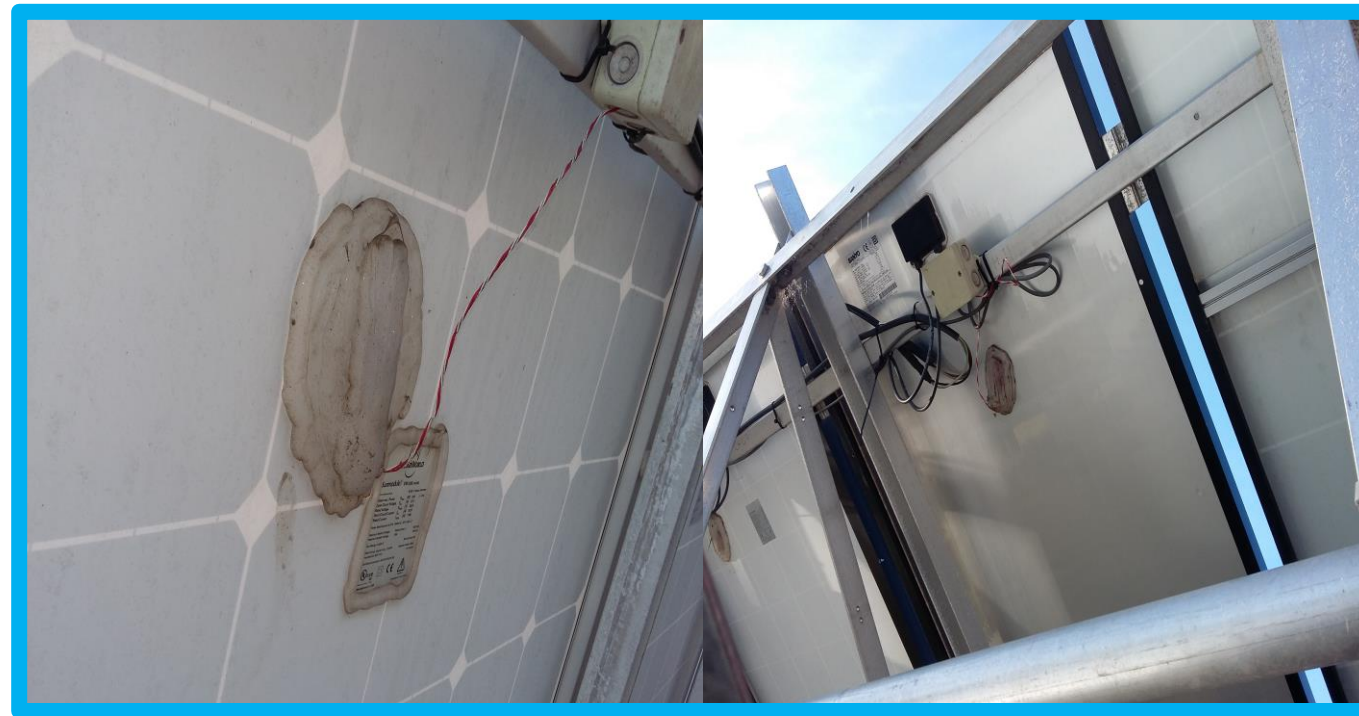
Fig. 4. Images of the BoM temperature fixation method used at the UK-LBOR test site.
