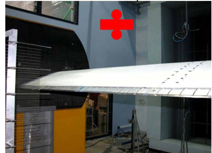
FIGURE C.2 THE TEST SECTION WITH THE TEST STAND AND THE WAKE RAKE DOWNSTREAM OF THE AIRFOIL SECTION.
