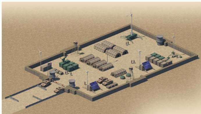
Rendering of a potential military or humanitarian base utilizing wind and solar as complements to diesel generation (Graphic courtesy of NREL)
