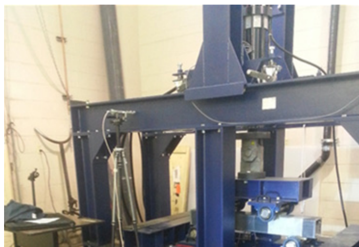
Montana State In-plane loader test frame for multi-directional fatigue testing. (Photo courtesy of Montana State University)
