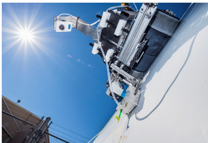
Sandia ARROWe NDI crawler robot. (Photo by Randy Montoya)
