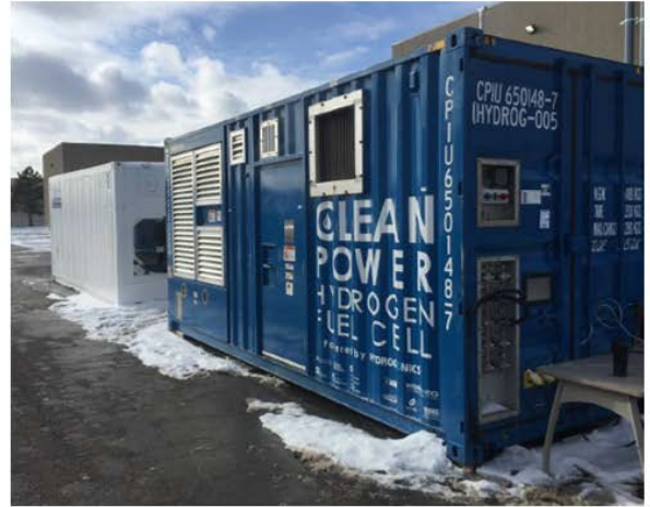
Figure 8. (L) Indoor testing of the MarFC unit at Cummins/Hydrogenics after system repair and upgrade; (R) outdoor testing of the MarFC unit in cold weather at the Cummins/Hydrogenics site in Mississauga, Ontario, Canada, December 2017.
