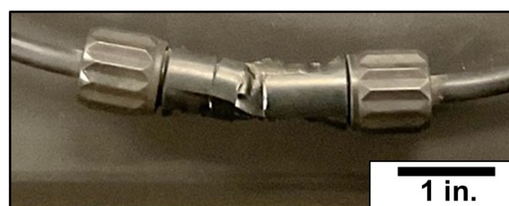
Fig.5 Example of a field-failed connector collected for forensic analysis
