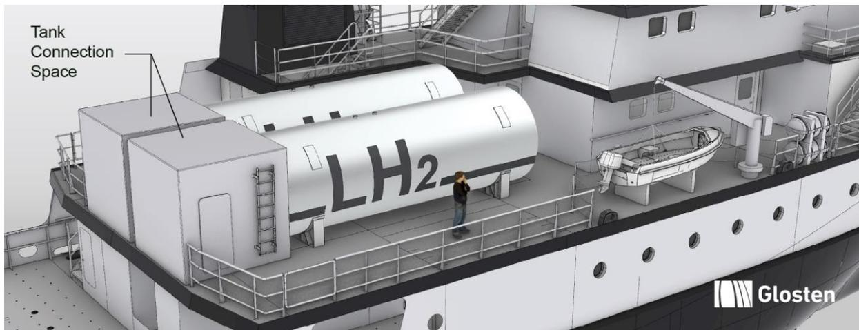
**Figure 12.** 3D rendering of H<sub>2</sub> Baseline Vessel LH<sub>2</sub> fuel tanks and tank connection spaces (TCSs).
