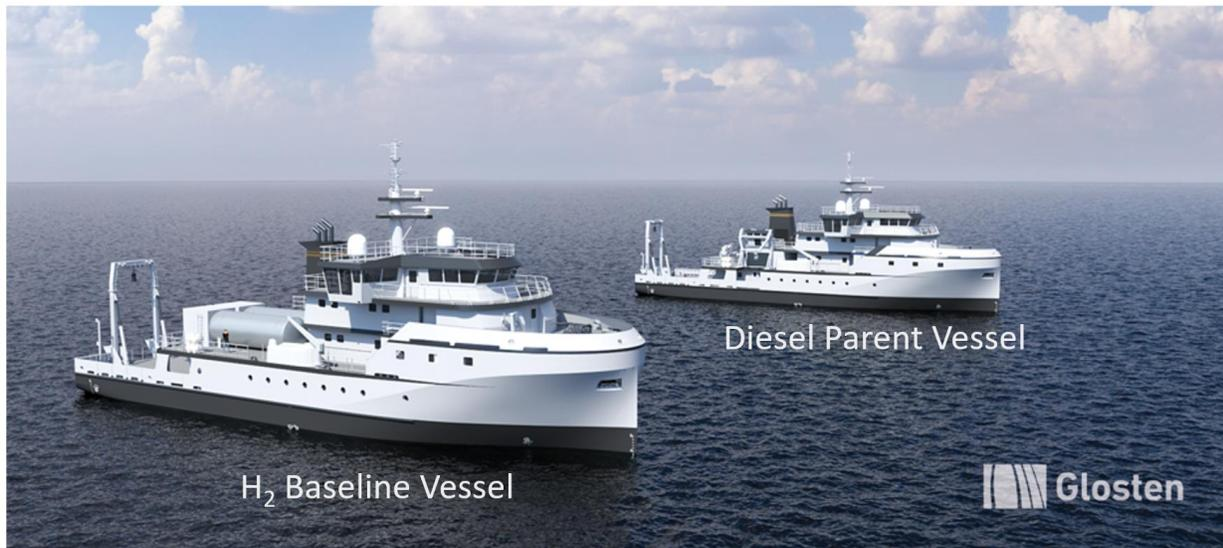
**Figure 22.** The 3D rendering of the H<sub>2</sub> Baseline Vessel used for comparison purposes in this study, along with a rendering of diesel-electric Parent Vessel from which the H<sub>2</sub> Baseline Vessel is derived.
