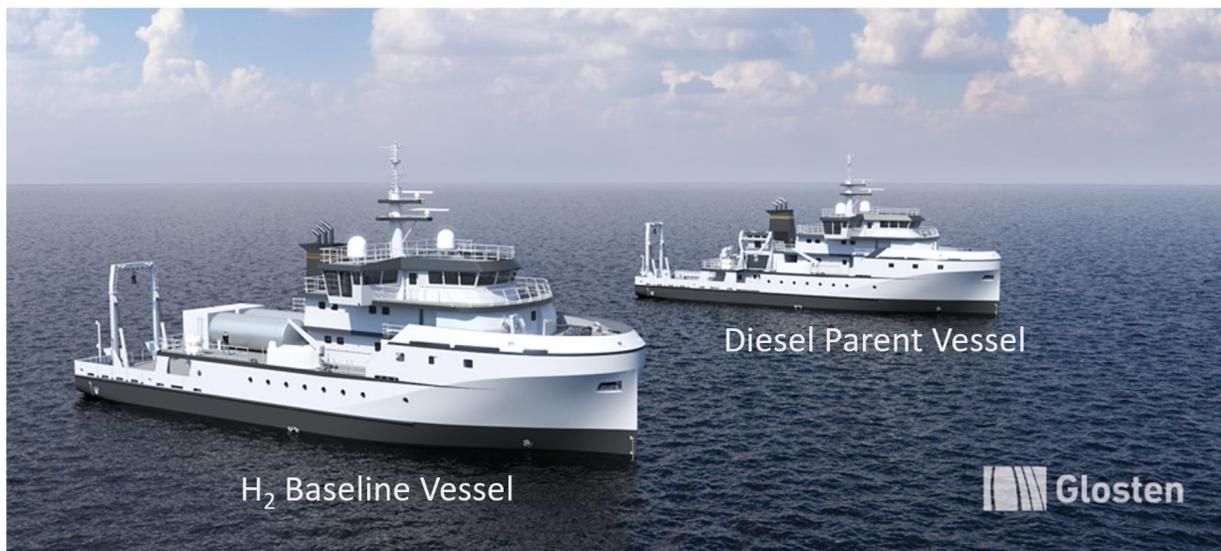
**Figure 9.** 3D renderings of H<sub>2</sub> Baseline Vessel and diesel-electric Parent Vessel from which the H<sub>2</sub> Baseline Vessel is derived.
