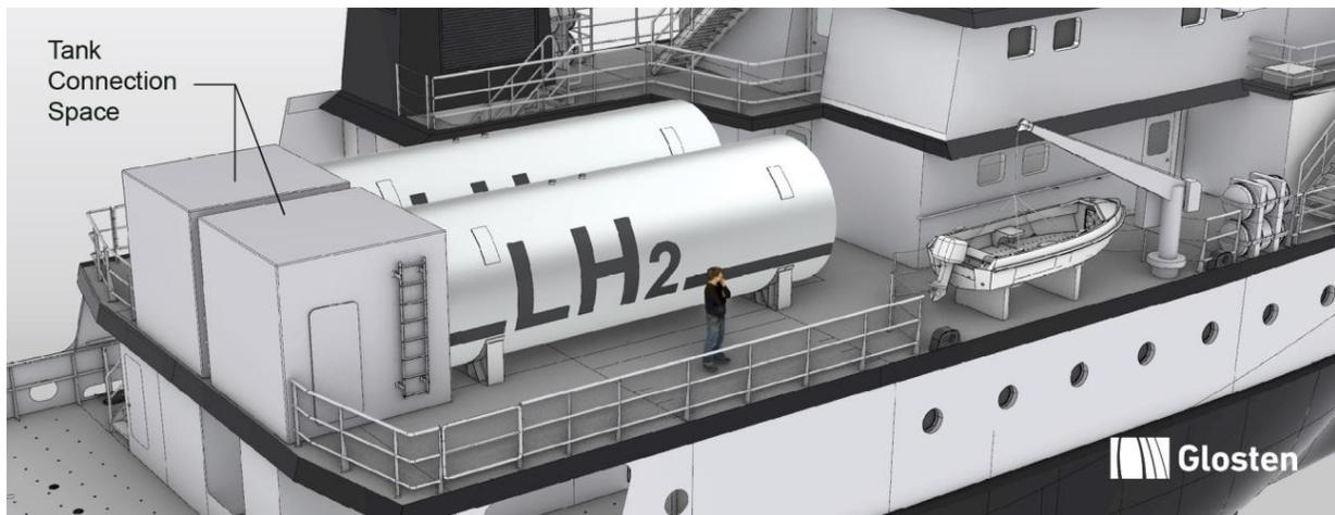
**Figure D.** 3D rendering of H<sub>2</sub> Baseline Vessel. LH<sub>2</sub> fuel tanks and tank connection spaces (TCSs) are indicated.
