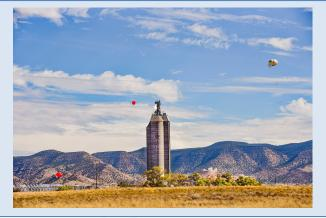
Three tethered balloons were deployed both upwind and downwind of Sandia National Laboratories' National Solar Thermal Test Facility during a falling-particle receiver test. The team found that the concentration of tiny particles, finer than talcum powder, that escape from the receiver were much lower than Environmental Protection Agency limits. (Photo by Randy Montoya)
