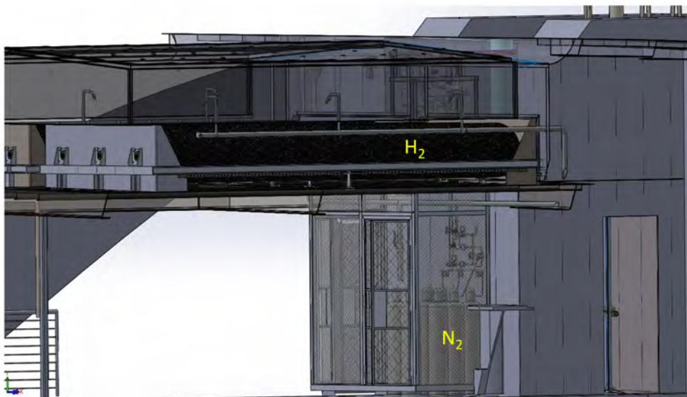
Figure 19: 3D model image of the nitrogen tanks providing gas pressure for operating pneumatic valves with the hydrogen technology system.
