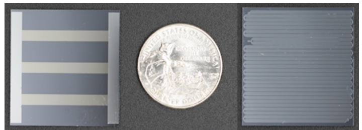
Figure 2. Sandia researchers are working to create a miniature, low-power universal greenhouse gas sensor using micro gas chromatography devices (left and right) about the size of a U.S. quarter (center).
