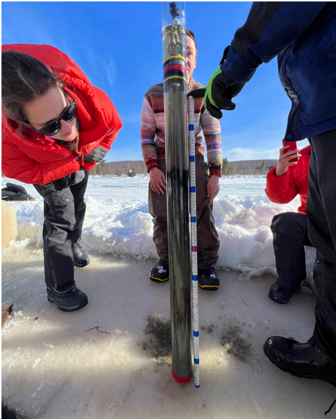
Sandia technologist Jenna Schambach inspects the sediment layers obtained in a 1-meter core from a frozen thermokarst lake bed at Big Trail Lake near Fairbanks, Alaska. Photo courtesy Chuck Smallwood.
