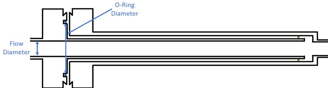
**Figure 26: Example schematic of a bayonet-style connector used in the transfer of liquid hydrogen**
