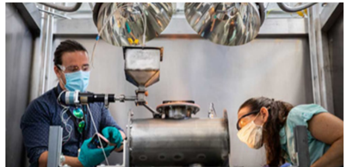
Sandia researchers have explored the use of concentrating solar thermal energy for low-carbon industrial ammonia production. Currently, conventional ammonia production accounts for roughly 1.5% of global CO 2 emissions.
