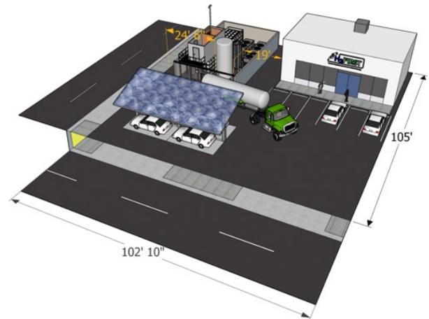
Hypothetical layout of hydrogen vehicle refueling station with compact layout using revised setback distances for liquid hydrogen in NFPA 2
