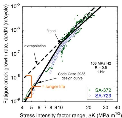
Fatigue crack growth rate design curves accepted into ASME Section VIII Division 3 Code Case 2938, [DOE Hydrogen Program of Record](#)
