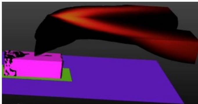
Example jet flame plume in a ventilated tunnel to determine fire damage on tunnel ceiling (Source: [SAND2017-11157](#))
